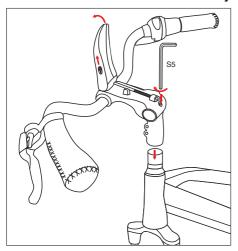
1. Open the top cover, align the stem with the head tube and slide it on. Tighten the screw at the top of the stem.
